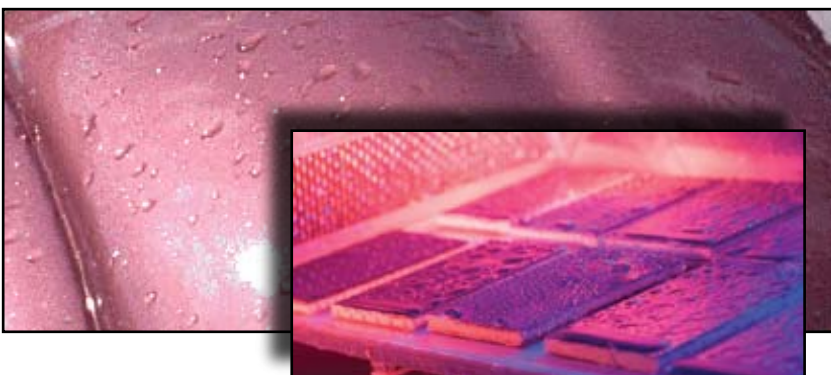
The Q-Sun's near-horizontal specimen orientation allows moisture to dwell on the surface of the test specimens to realistically reproduce the natural outdoor exposure conditions of many materials.
