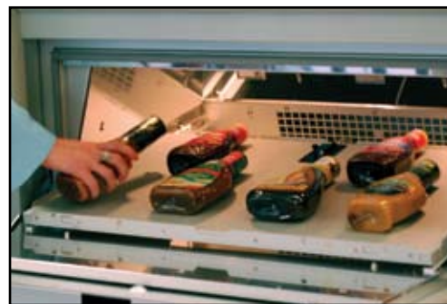
3-D specimens can be placed directly on the specimen tray and in most cases do not require a specimen holder.
