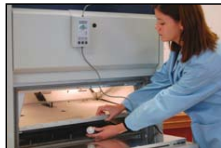
The CR20's UV sensor is placed into the calibration port located in the specimen tray.
