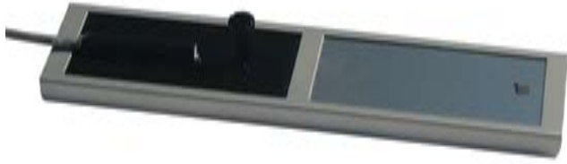
The Black Panel Temperature sensor is mounted in a 2x4" specimen holder.
