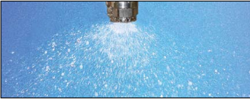
The Q-Sun uses a pure water spray to simulate outdoor moisture attack.
